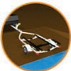
Pull trailer out of water and away from the ramp.
