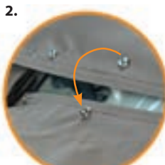
2. Overlay cockpit cover and begin snapping all windshield snaps
